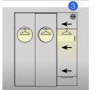
When any door is open, the light turns on.
